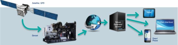
Teksan Remote Monitoring and Management System, supported by GSM and internet technologies, is a highly useful and cost-effective web-based solution that allows remote generator monitoring and intervention when needed. This system, which has the latest technologies, sends the working data of the generator on the field via the control panel to a remote device such as a computer, tablet or smartphone and allows the generator to be managed via this device.
